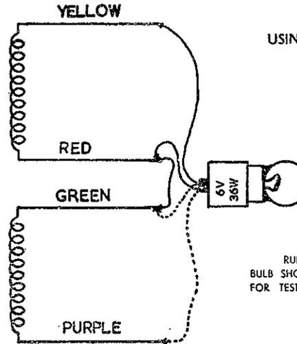
USING A 6 VOLT 36 WATT BULB
