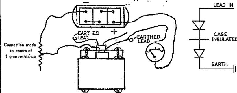
CONNECT BATTERY + VE THROUGH 'AMMETER TO EARTH TAG AND BATTERY - VE THROUGH 1 OHM RESISTANCE TO FREE LEAD OF RECTIFIER. CURRENT 10 AMPS. (approx). REVERSE BATTERY CONNECTIONS CURRENT LESS THAN 100 MILLIAMPS. REPEAT FOR THE OTHER RECTIFIER.
